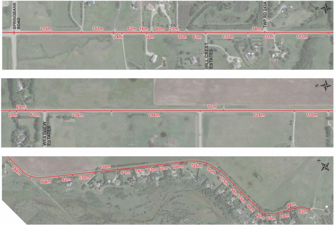
Figure 2: Existing Access Spacing on Range Road 33
